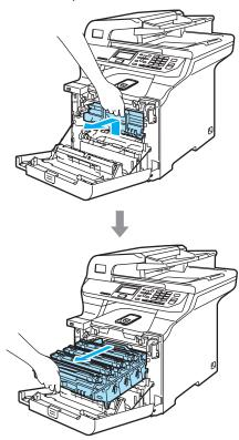
Release the gray lock lever (1) that is on the left side of the machine. Lift the front of the drum unit and pull the drum unit completely out of the machine using the green handles on the drum unit.
